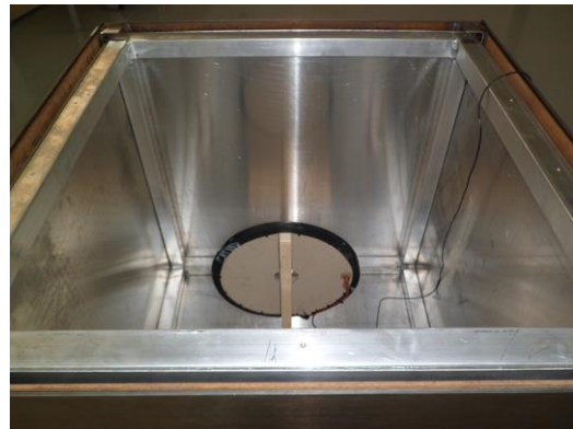
Figure 4. Transmission loop antenna inside of aluminium enclosure.
