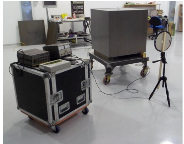
Figure 5. Shielding Set up measurements of the two enclosures.
